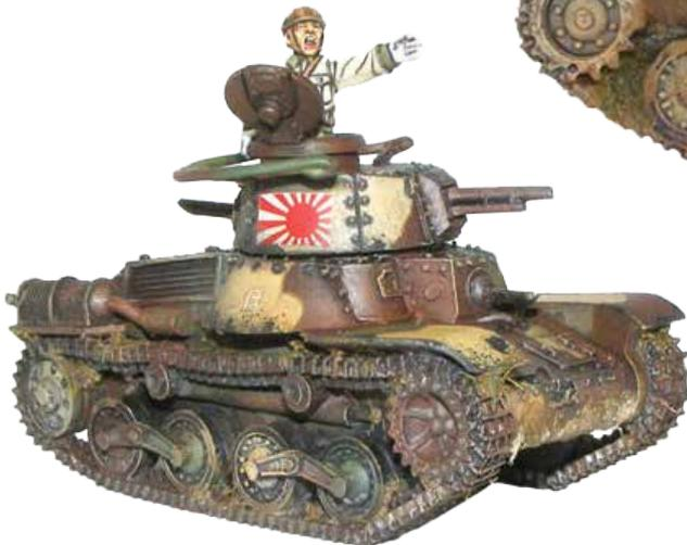
◀When the Imperial Japanese Army replaced the turrets on the Type 97 Chi-Ha medium tanks - creating the Type 97 ShinHoTo - the original turrets were retro-fitted to the obsolete Type 95 Ha-Go light tanks. These were designated the Type 4 Ke-Nu. This example here has a lighter ochre colour than ours, has been painted without the wavy yellow lines, and displays a very prominent Rising Sun on the turret.
